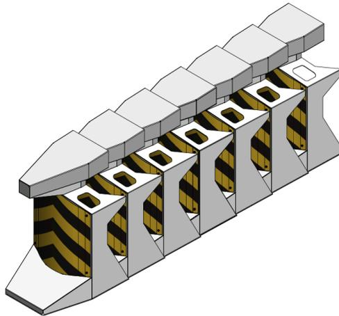
Figure 4.4: Recommended Storage and Transportation Method for Quash™ Nose Piece
