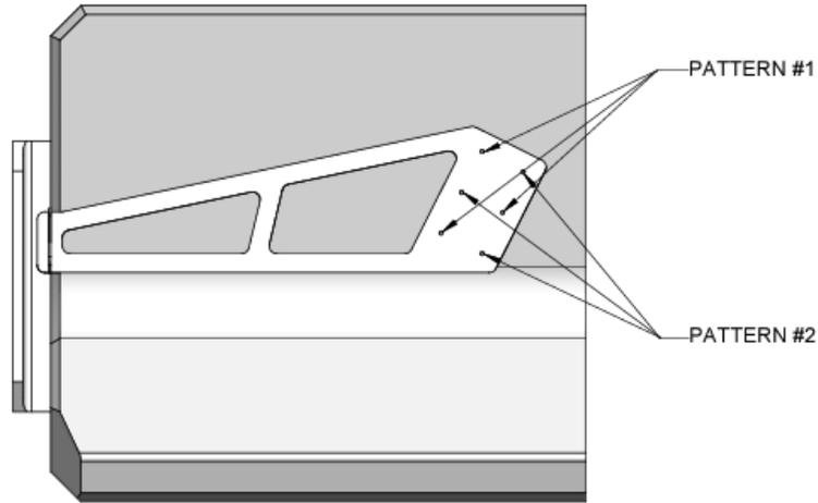
Figure 5.2.4: Quash™ Jigging tool on Barrier
