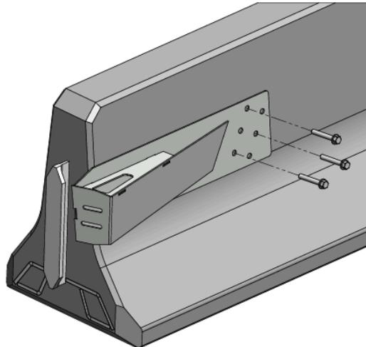
Figure 5.2.5: Quash™ Left Transition on Barrier Anchoring
