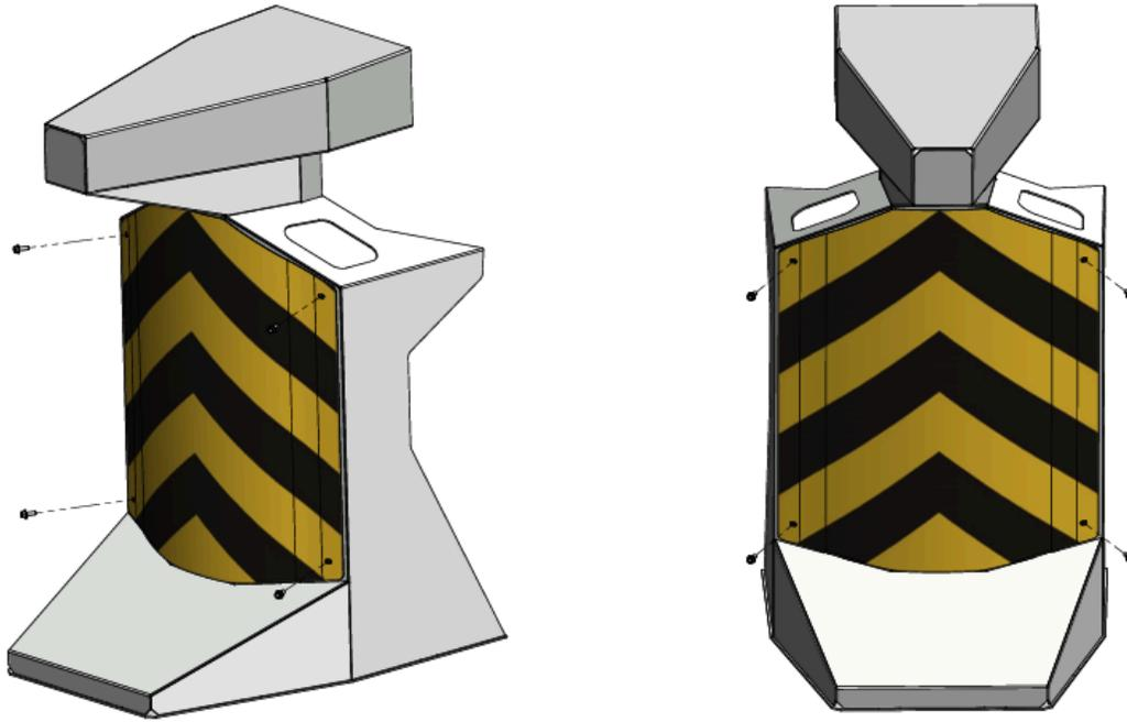
Figure 5.4.1: Quash™ Nose Piece Delineation Panel Installation
