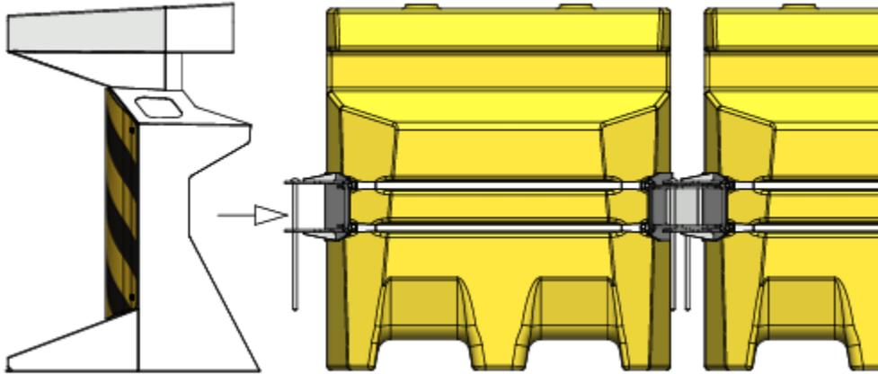
Figure 5.4.2: Quash™ Nose Piece Assembly on First Cell
