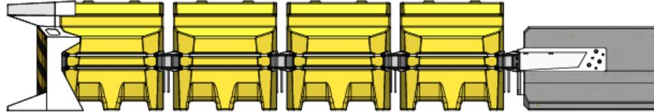
Figure 2.2: Quash™ Crash Cushion Configuration Arrangement for TL-2
