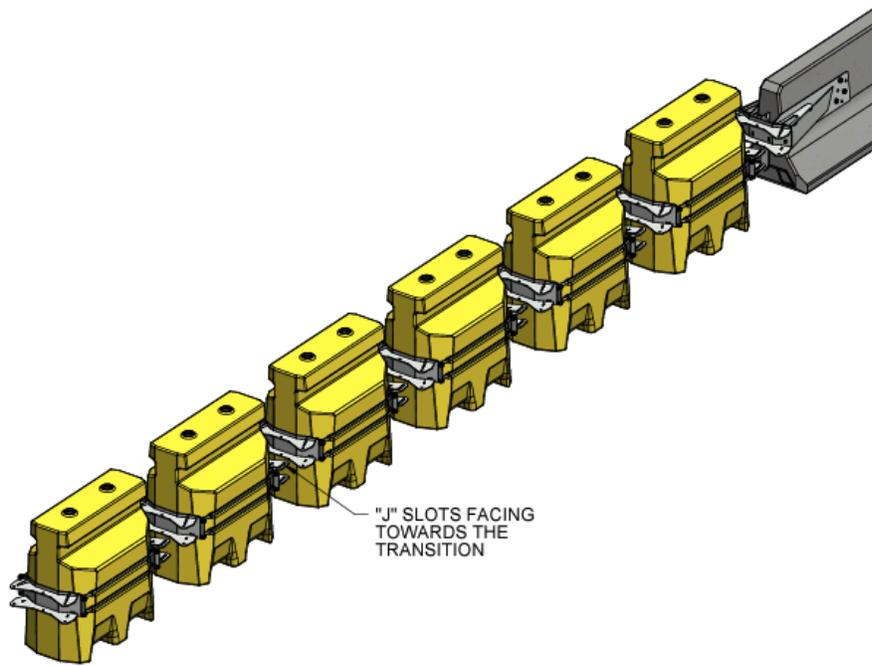
Figure 5.3.1: Installation of Quash™ Cells for TL-3 Configuration
