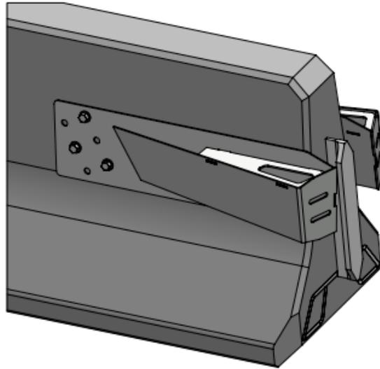
Figure 5.2.6: Quash™ Left and Right Transition on Barrier
