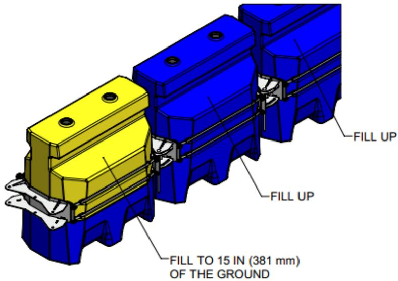
Figure 5.3.8: Quash™ TL-2 Configuration: First Cell: Fill to 15 in. from Ground Level
