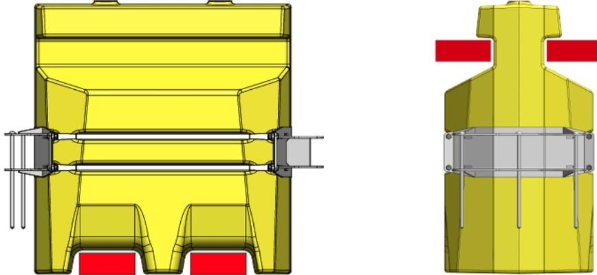
Figure 4.1: Recommended Lifting Methods for Quash™ Absorption Cells
