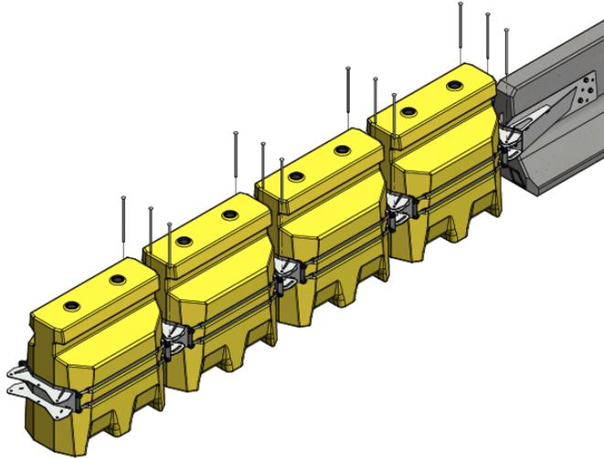
Figure 5.3.4: Installation of Quash™ Pins on Barrier for the TL-2 Configuration
