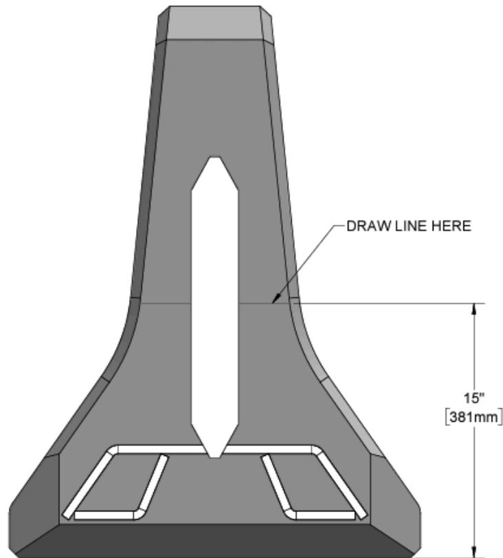
Figure 5.2.1: Quash™ Line on Barrier, 15 in. from the Ground
