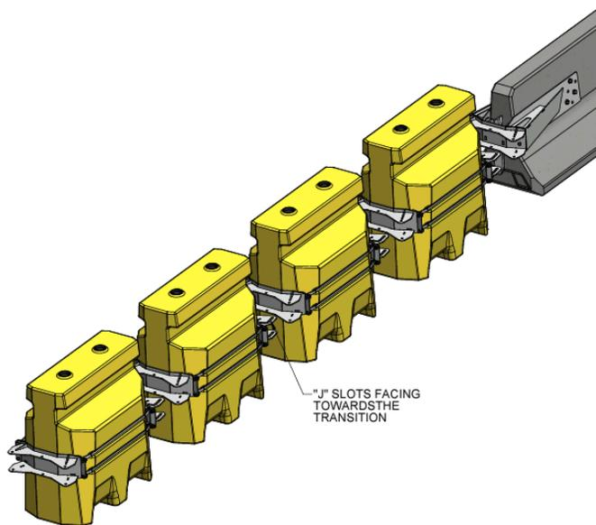
Figure 5.3.2: Installation of Quash™ Cells for TL-2 Configuration
