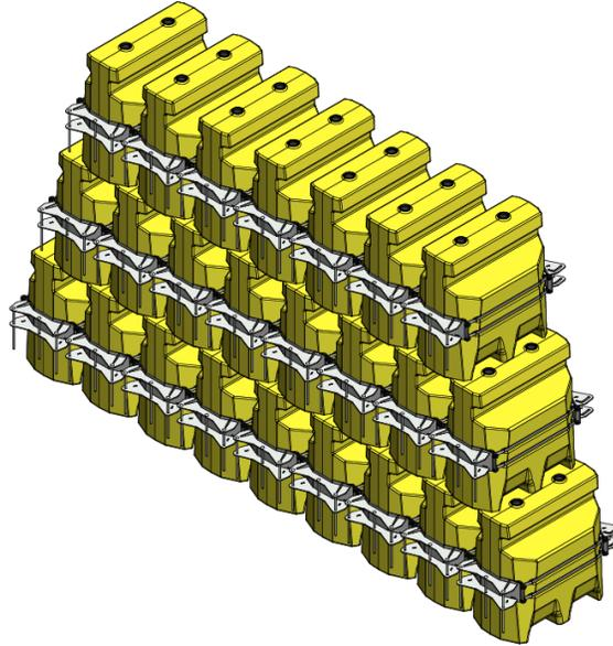
Figure 4.3: Recommended Storage Method for Empty Quash™ Absorption Cells
