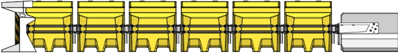
Figure 2.1: Quash™ Crash Cushion Configuration Arrangement for TL-3
