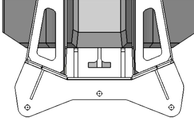
Figure 5.2.8: Quash™ Transition Front Plate Stoppers Resting on the Front of the Barrier
