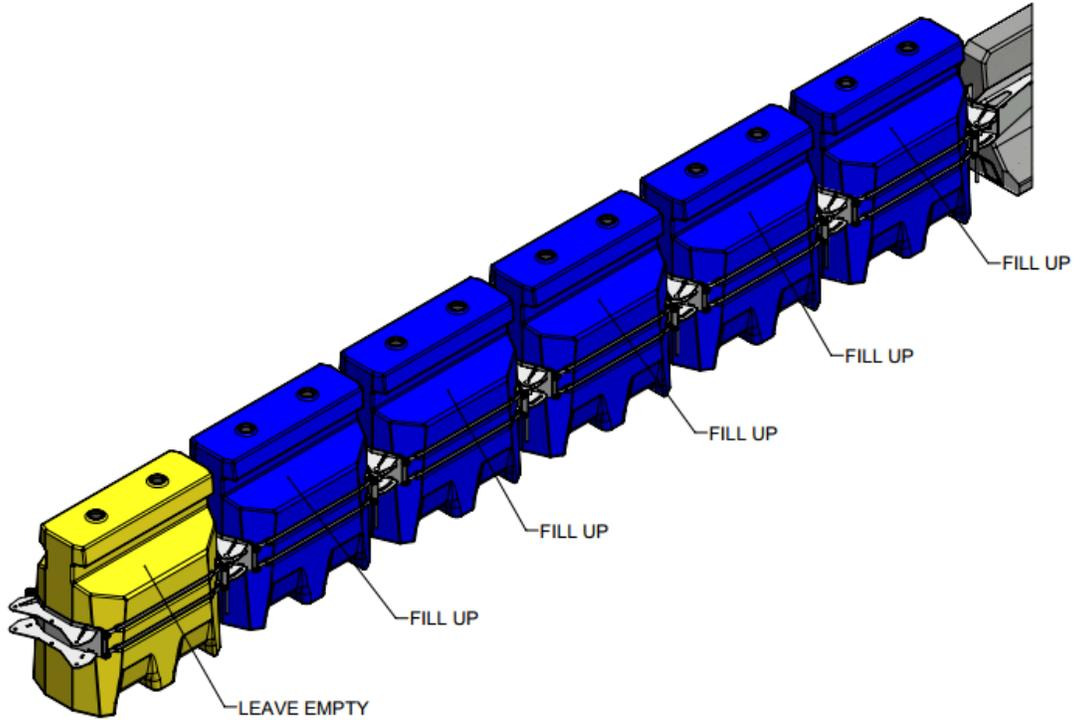
Figure 5.3.7: Filling Cells for the Quash™ TL-3 Configuration
