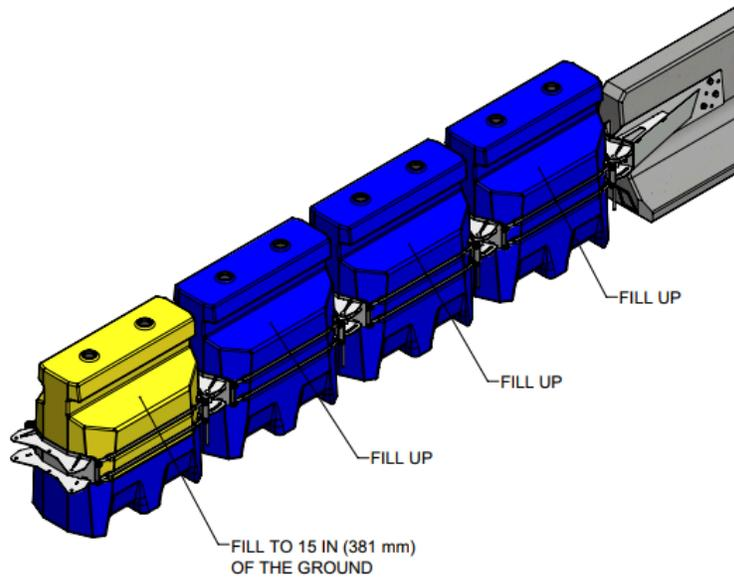
Figure 5.3.9: Filling Cells for the Quash™ TL-2 Configuration
