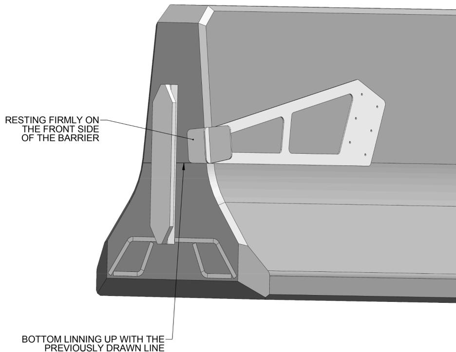
Figure 5.2.3: Quash™ Jiggling Tool on Barrier
