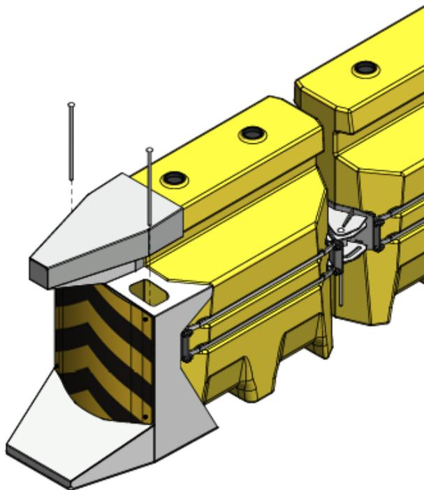
Figure 5.4.3: Quash™: Securing Nose Piece to First Cell with Pins
