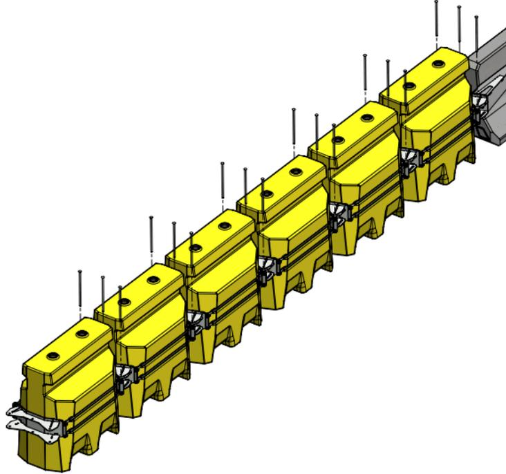
Figure 5.3.3: Installation of Quash™ Pins on Barrier for the TL-3 Configuration
