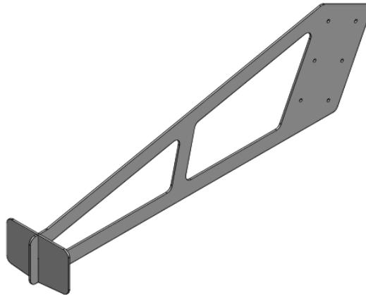
Figure 5.2.2: Quash™ Transition Jiggling tool (Part #: Q600-100012-000)
