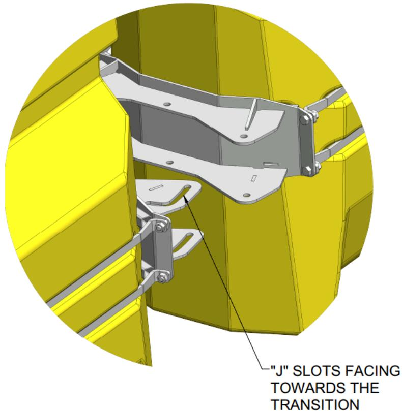
Figure 5.3.0: Quash™ Cell Orientation during Installation
